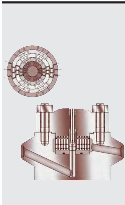
Fig. 14. MIL 78000. Reheater Attenuator Control Valve.
